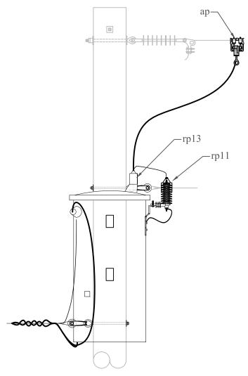
Note: Install item "fo" if service weather head or service take-off is more than 12 inches below bottom of transformer can.
